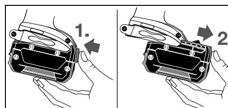
To remove the battery **8**, press the unlocking button **9** and pull out the battery toward the front. **Do not exert any force**
