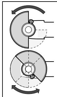
Place the protection guard **7** on the spindle collar. Adapt the position of the protection guard **7** to the requirements of the work step. Lock protection guard **7** by tightening locking screw **8** with combination spanner **4**.
